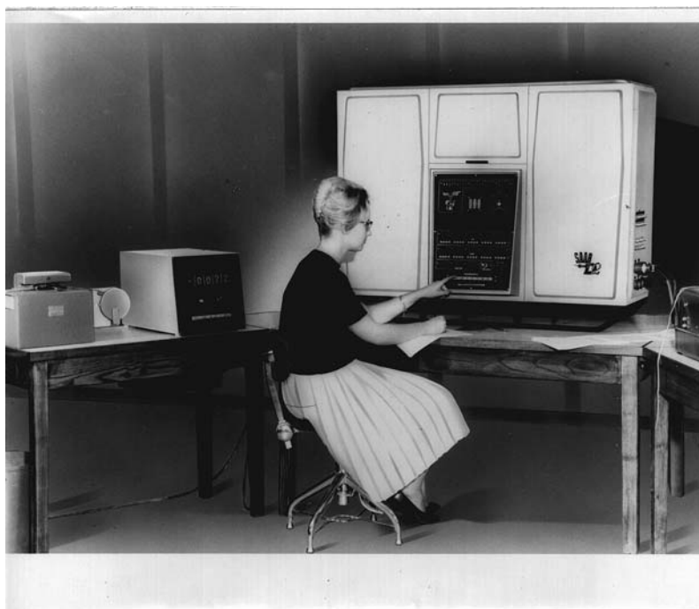
Figure 2, Computer Saab SANK/D2 with strip reader, punch, digital display and the operator.
